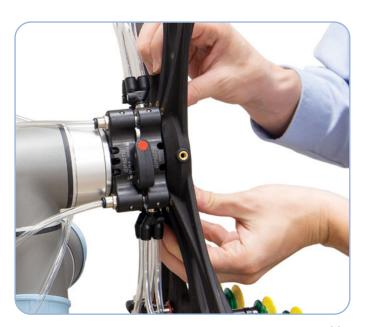
With the same mounting pattern as the tool flange of your cobot (ISO-9409-1-50-4-M6), you can mount any "Plug & Play" end effector to the QC75-B for a quick and repeatable installation for every job. End effectors can be hard-wired to the QC75-B, or plugged to the wrist connector of your Cobot for even faster setup times.
