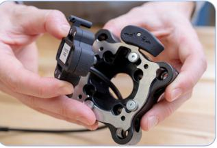
Replace the Electrical Connector back into the QC75 and fasten with same hardware. Note that cables are meant to run down the backside grooves of the QC75 to avoid any cables from pinching.
