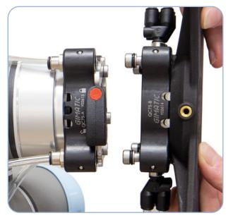
Designed for collaborative robots, the QC75 is a manual quick changer that allows for pneumatic and electrical connections to be easily coupled between jobs. Standardize up to 16 electrical contacts and 4 pneumatic lines to have your cobot up and running with minimal downtime.
