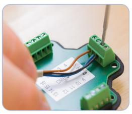
(16x) Screw terminals allow you to standardize on tools with a single sensor or various electric grippers or valves.
